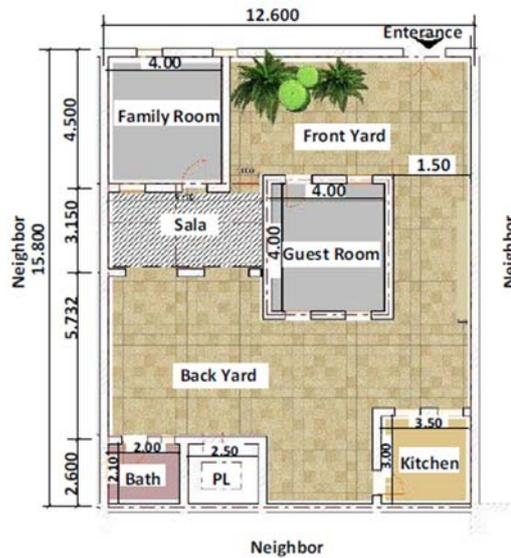
Figure (2) plan of the core unit - New Deims.
