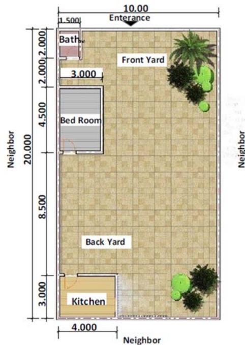
Figure (5) plan of the core unit - Elthora hara 72.
