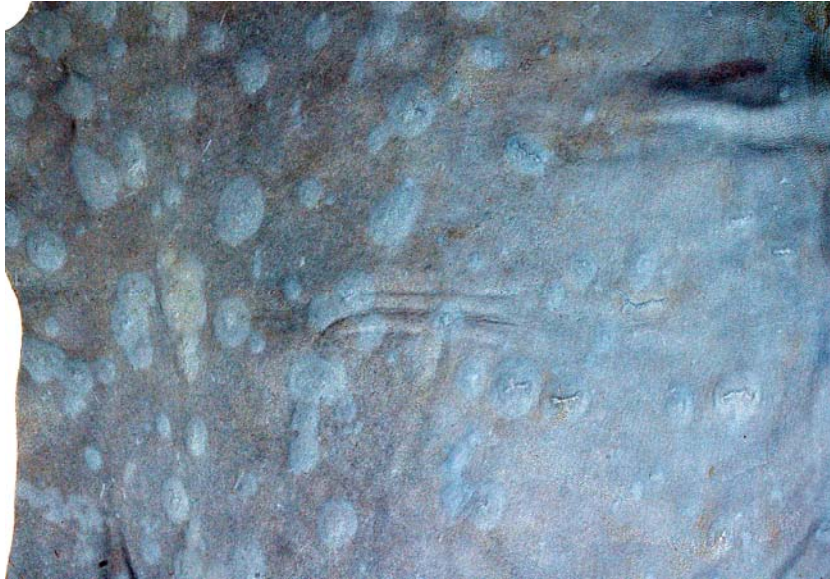
Plate (1) Bacterial damage-wet blue hides
