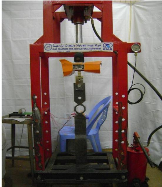
Figure (7). Calibration setup of drawbar transducer
